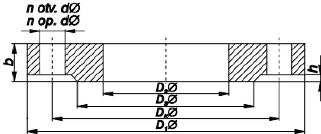
**NOTE:** The connection dimensions correspond to the SRPS M.B6.011 and DIN 2501 standard, and the quality of the material or the thickness of the flanges is determined by calculation.
