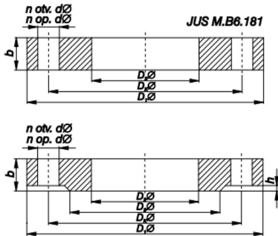
**NOTE:** Up to DN 700 flanges comply with the SRPS M.B6.181 standard. Other sizes of flanges have connection dimensions according to SRPS M.B6.011 and DIN 2501 standards, and the quality of the material or the thickness of the flanges is determined by calculation.
