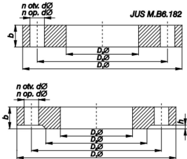
**NOTE:** Up to DN 700 flanges comply with the SRPS M.B6.182 standard. Other sizes of flanges have connection dimensions according to SRPS M.B6.011 and DIN 2501 standards, and the quality of the material or the thickness of the flanges is determined by calculation.
