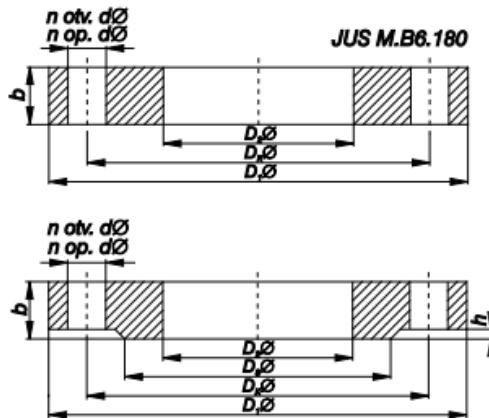
**NOTE:** Up to DN 800 flanges comply with the SRPS M.B6.180 standard. Other sizes of flanges have connection dimensions according to SRPS M.B6.011 standards, and the quality of the material or the thickness of the flanges is determined by calculation.
