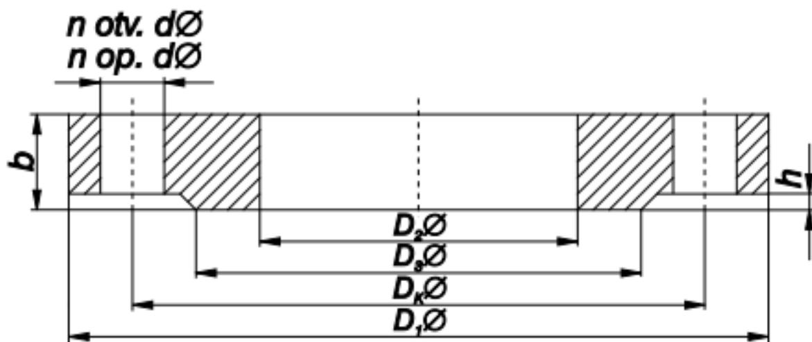
**NOTE:** The connection dimensions correspond to the SRPS M.B6.011 and DIN 2501 standards, and the quality of the material or the thickness of the flanges is determined by calculation.
